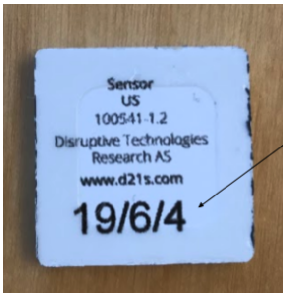
Figure 1: Picture of position of PN 100543 DT Node0 Backside Graphics, US. The print is located on the backside of the sensor.
