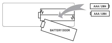
Remove the battery compartment cover on the back of your remote by carefully sliding to open. The battery cover can then be lifted away. Fit the correct batteries (2 X AAA batteries not included), referring to the polarity markings. Finally, replace the cover.
