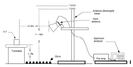
Above 18 GHz shall be extrapolated to the specified distance using an extrapolation factor of 20 dB/decade form 3m to 1m.
