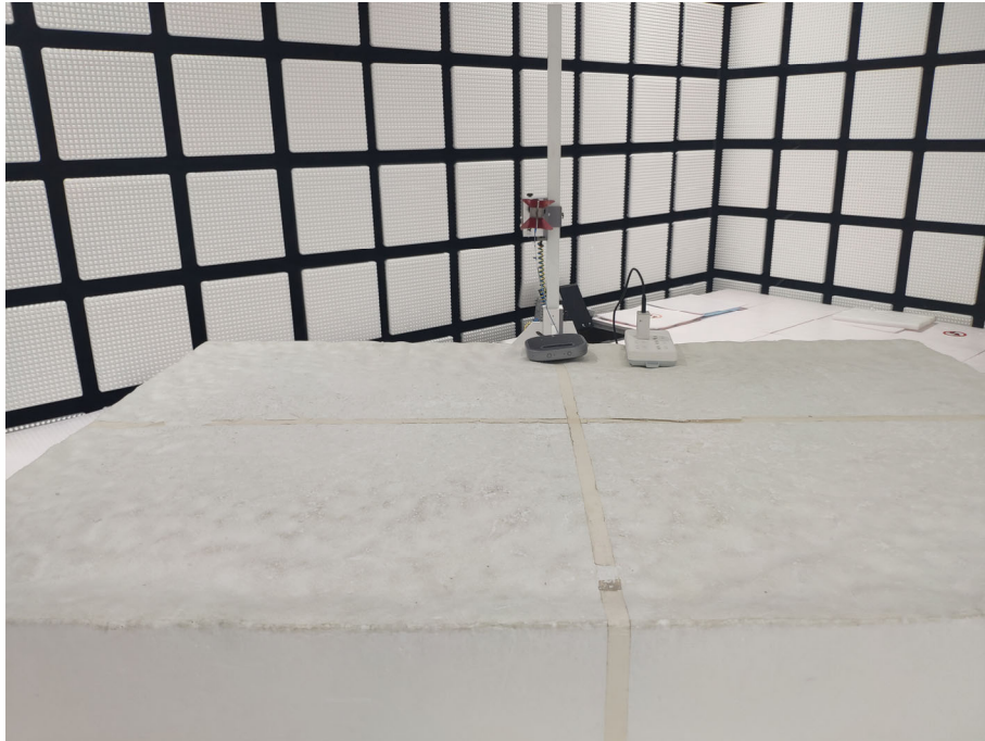
Radiated spurious emission Test Setup-2(Above 1GHz)
