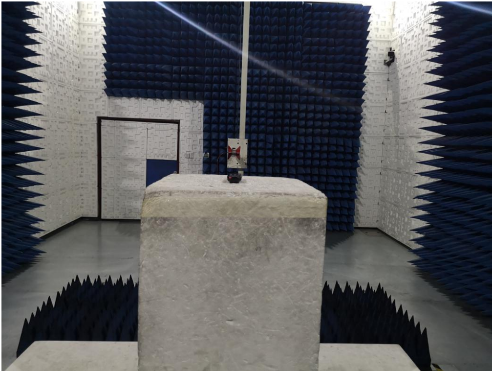
RADIATED EMISSION TEST SETUP ABOVE 1GHZ
