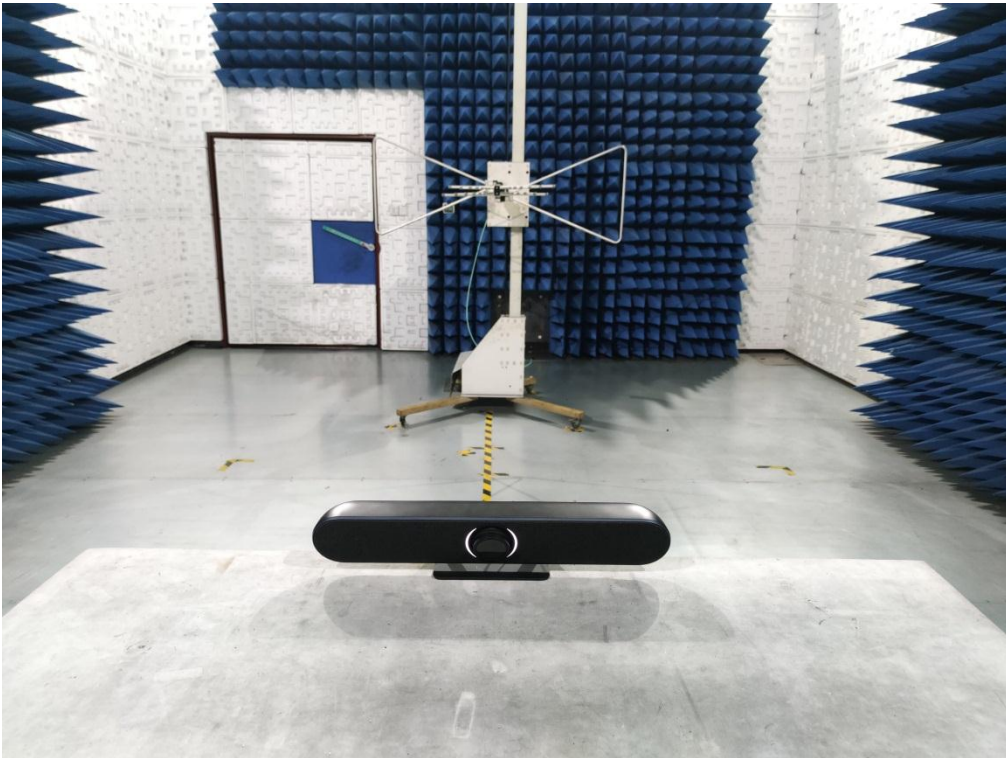
RADIATED EMISSION TEST SETUP ABOVE 1GHz
