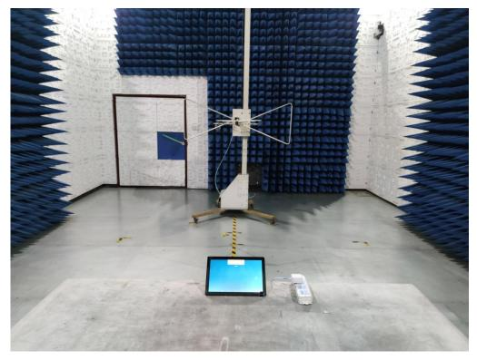
RADIATED EMISSION TEST SETUP ABOVE 1GHZ
