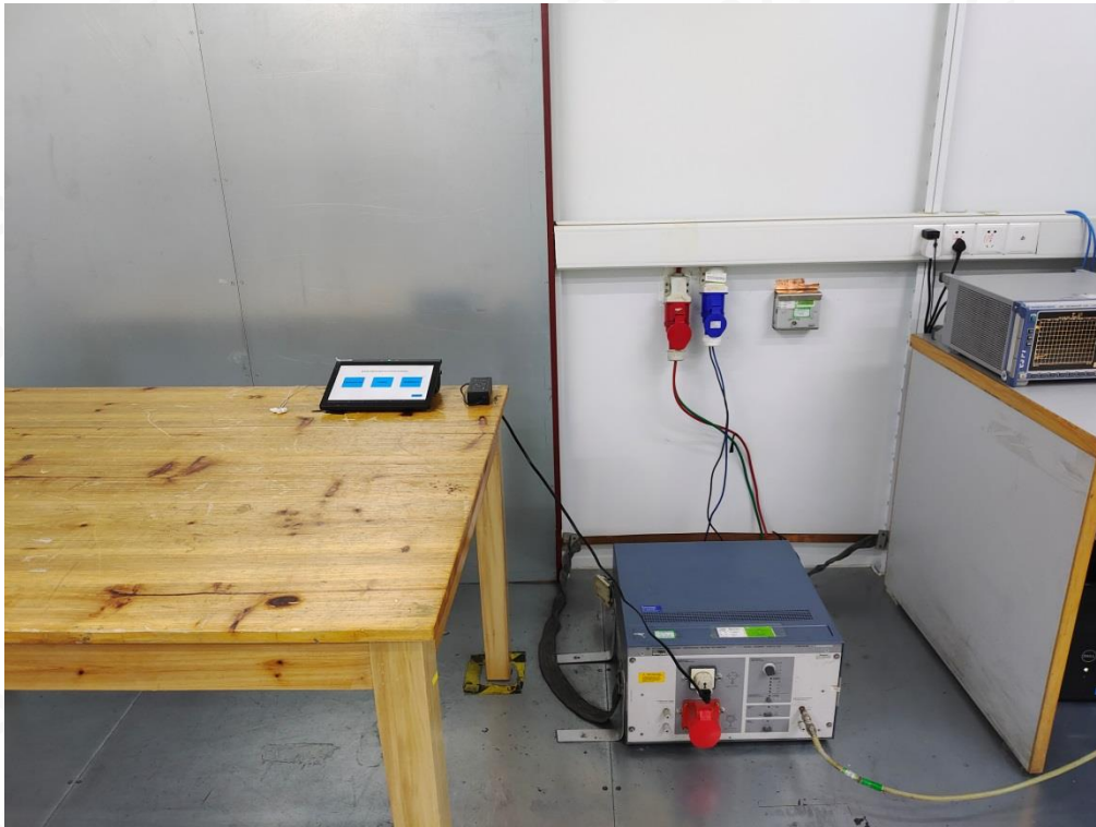
RADIATED EMISSION TEST SETUP BELOW 1GHZ
