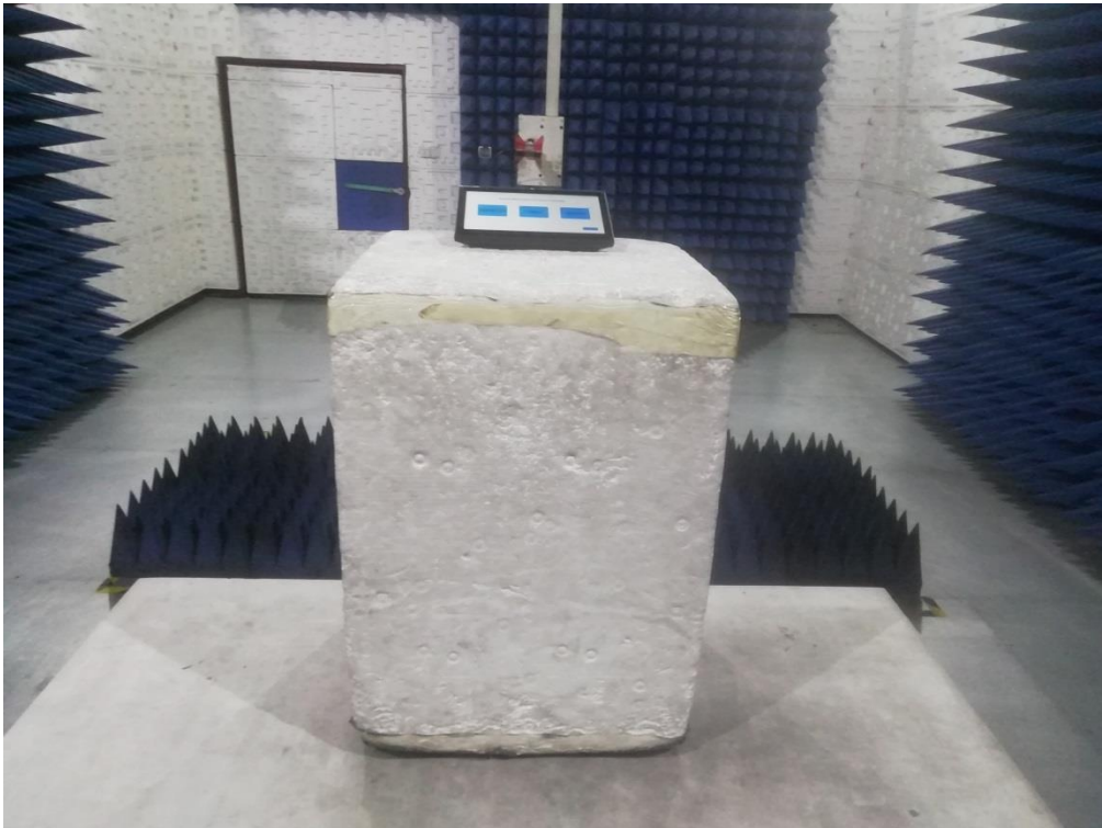
RADIATED EMISSION TEST SETUP ABOVE 1GHZ
