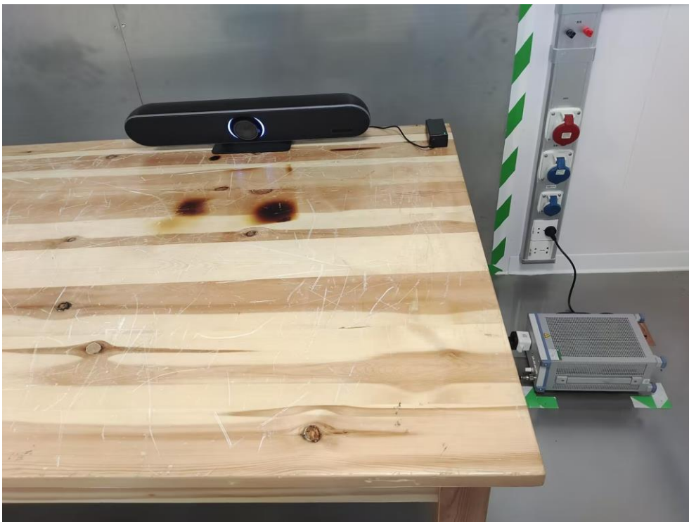
Power Line Conducted Emission
