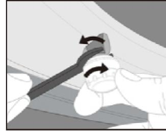
3. Hold the sensor, tighten Anti-theft screw
