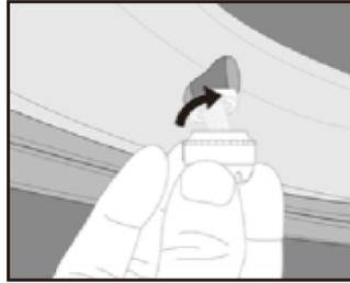
2. Install outer sensor on tire valve in order
