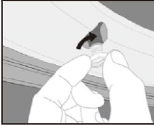
1. Remove tire valve cap, put in Anti-theft screws
