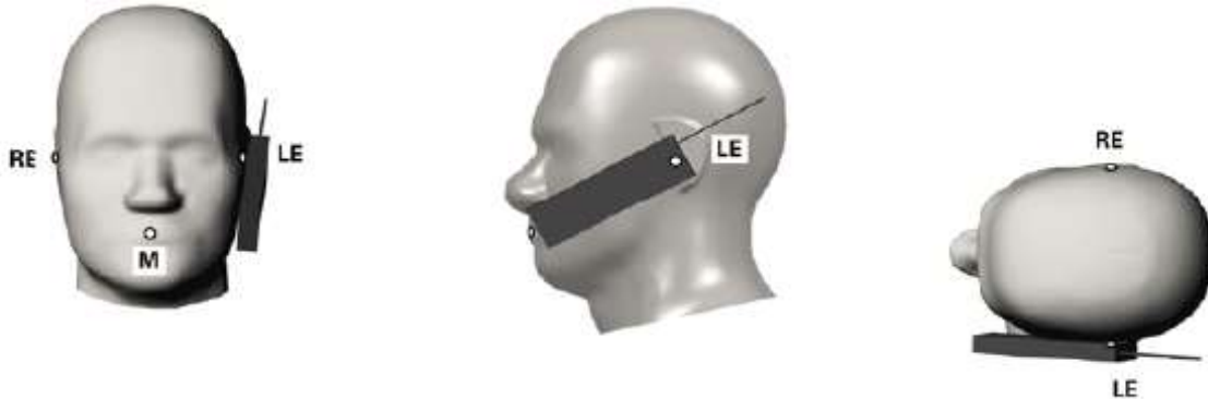
Fig. 11.3 Illustration for Cheek Position
