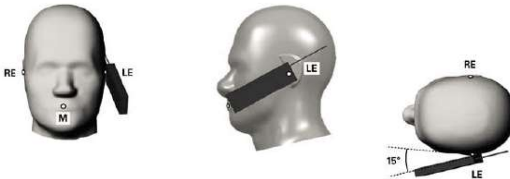
Fig.11.4 Illustration for Tilted Position
