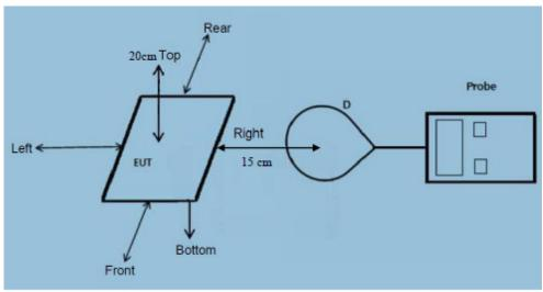
Remark: The EHP 200A probe antenna diameter is less than 11.5cm.
