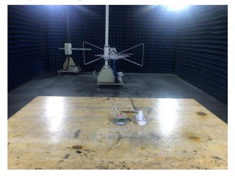
Photograph 3: Set-up for Radiated Spurious Emission,30MHz - 1GHz
