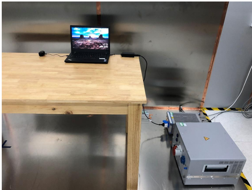
Photograph 4: Set-up for Radiated Emissions, below 1GHz mode B
