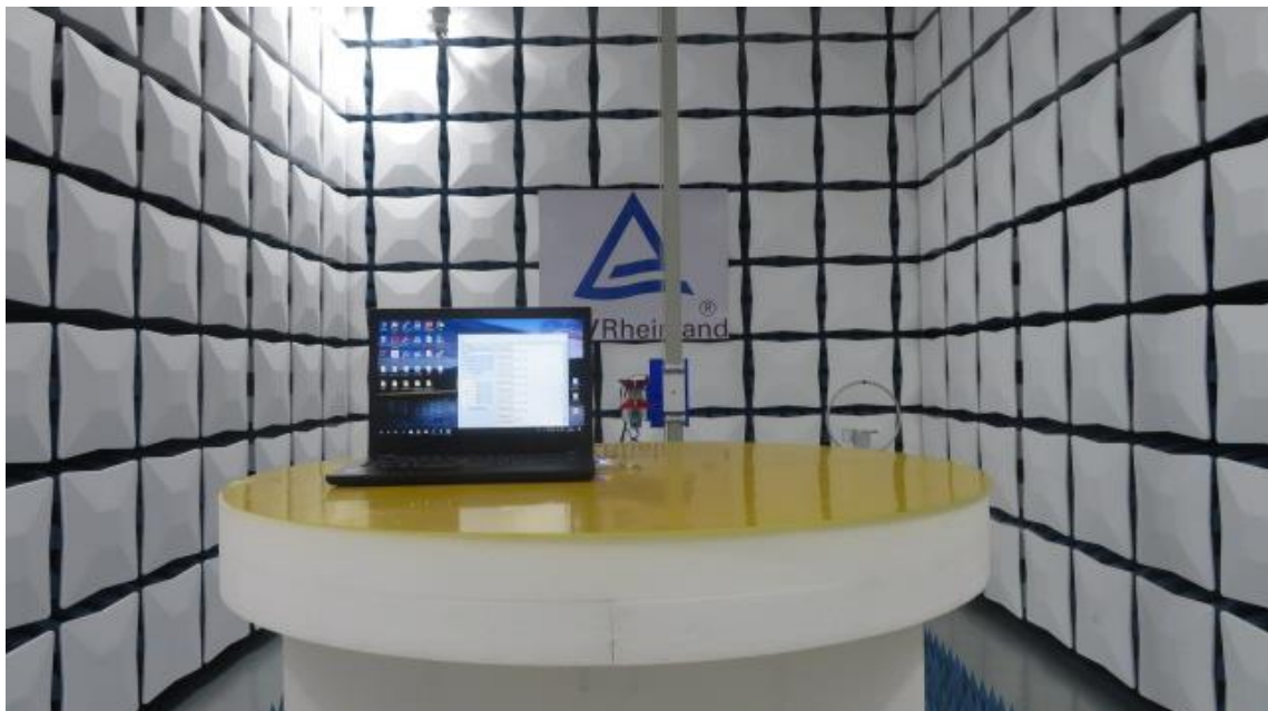
Photograph 2: Set-up for Spurious Emissions (1GHz-18GHz)
