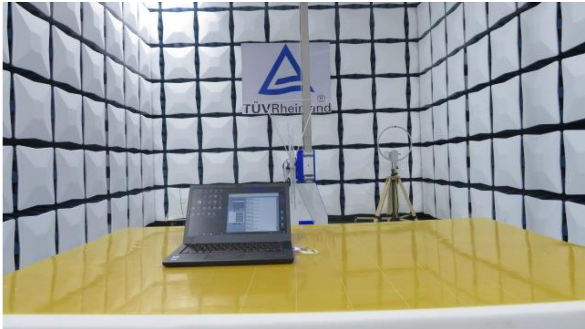
Photograph 2: Set-up for Spurious Emissions (1GHz-18GHz)
