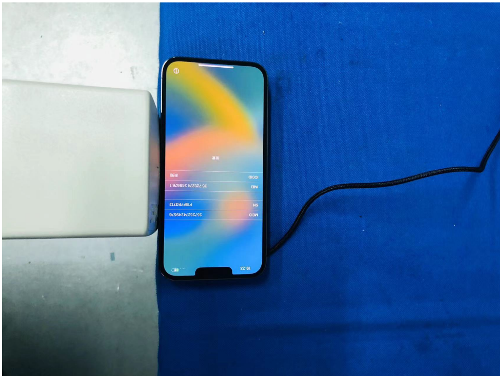
Photograph 4: Set-up for RF Exposure
