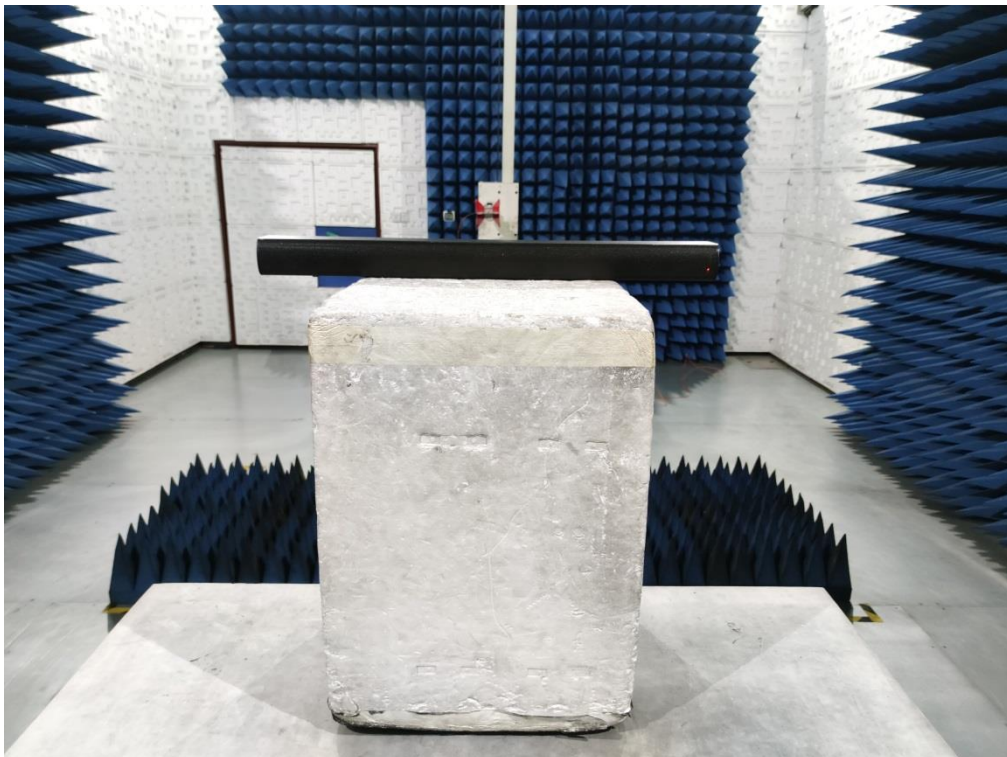
RADIATED EMISSION TEST SETUP ABOVE 1GHz
