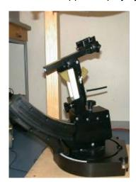
The DASY device holder is constructed of low-loss POM material having the following dielectric parameters: relative permittivity  $\epsilon$ =3 and loss tangent  $\sigma$ =0.02. The amount of dielectric material has been reduced in the closest vicinity of the device, since measurements have suggested that the influence of the clamp on the test results could thus be lowered.
