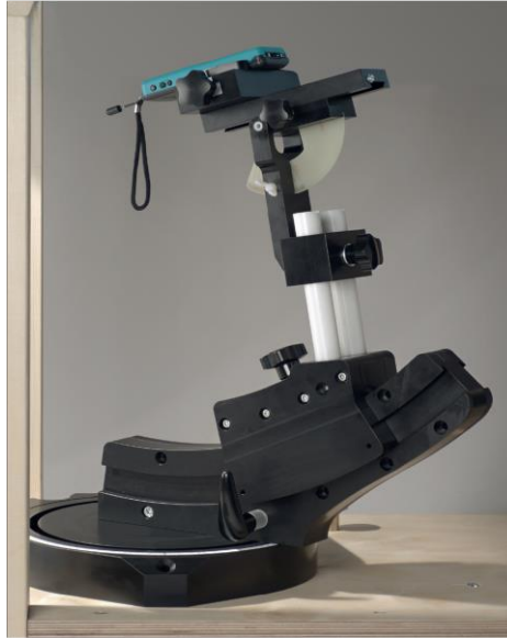
F-2. Device Holder for Transmitters
