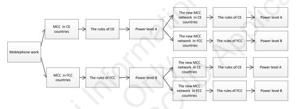
The software of the device has information of CE and FCC countries so that to detect where the users are. If the users are in CE countries, the power level A is applied. If the users are in FCC countries, the power level B is applied.
