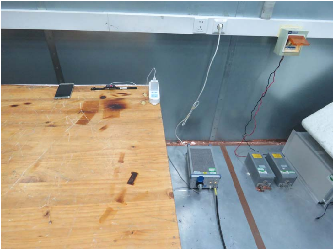
Picture 2: Conducted Emissions Test Setup
