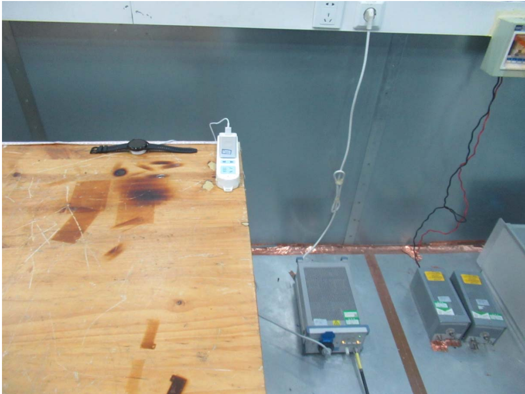
Picture 2 Conducted Emission Test Setup
