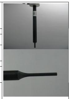
Isotropic E-Field Probe EX3DV4 for Dosimetric Measurements
