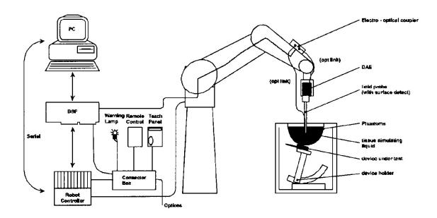
The DASY system for performing compliance tests consists of the following items:
