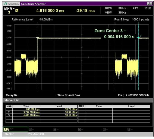
The duty cycle plot is shown above, so the duty cycle of bluetooth is calculated as below:
