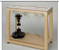
The bottom plate contains three pairs of bolts for locking the device holder. The device holder positions are adjusted to the standard measurement positions in the three sections.
