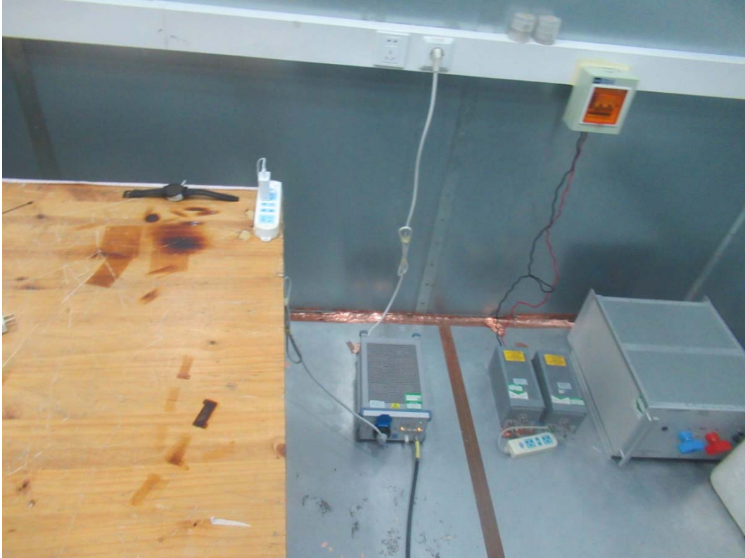
Picture 2: Conducted Emissions Test Setup
