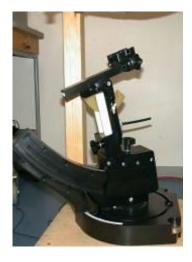
The DASY device holder is constructed of low-loss POM material having the following dielectric parameters: relative permittivity  $\varepsilon$ =3 and loss tangent  $\sigma$ =0.02. The amount of dielectric material has been reduced in the closest vicinity of the device, since measurements have suggested that the influence of the clamp on the test results could thus be lowered.
