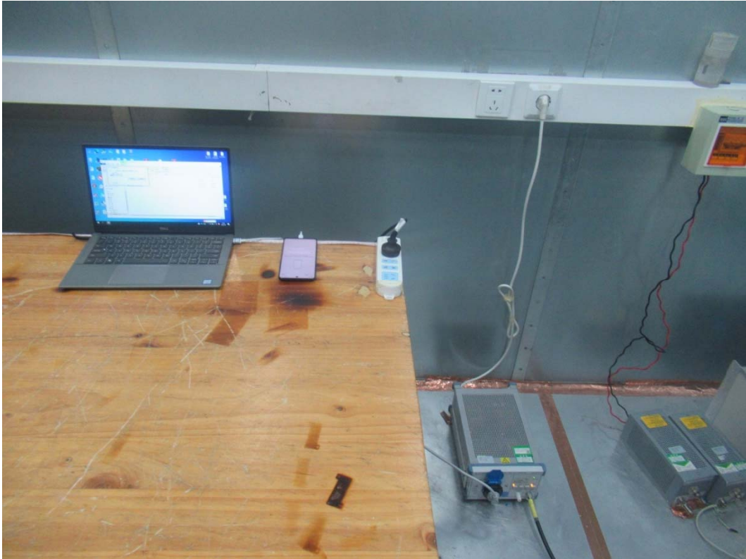
Picture 2: Conducted Emissions Test Setup
