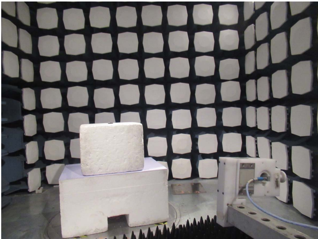
Picture 1 Radiated Emission Test Setup
