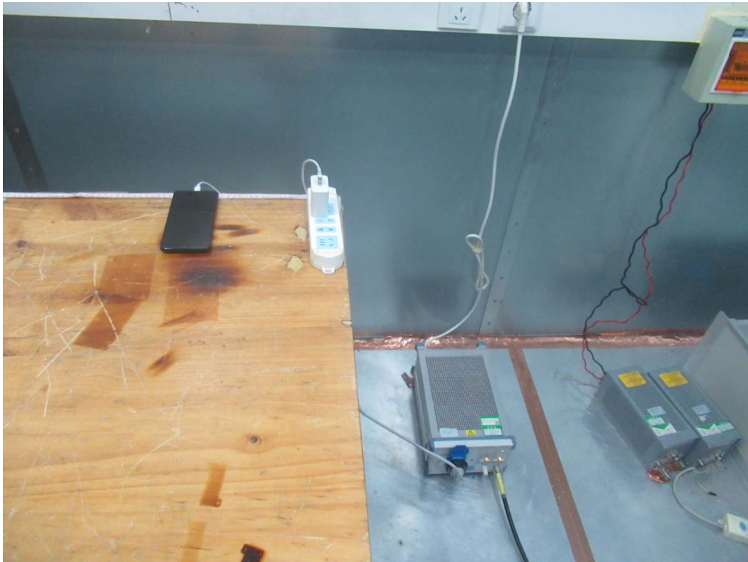
Picture 2 Conducted Emission Test Setup
