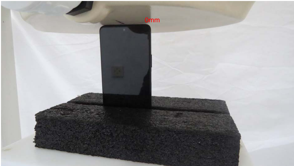
Picture 15: Top Edge, the distance from handset to the bottom of the Phantom is 0mm
