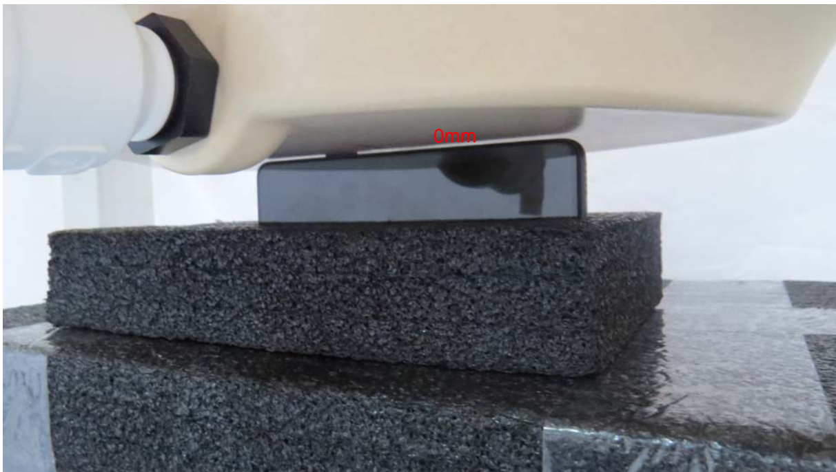
Picture 18: Right Edge, the distance from handset to the bottom of the Phantom is 0mm
