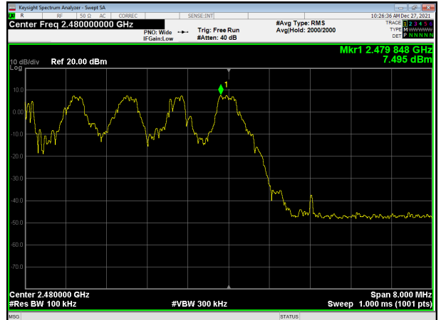
BT DH5 CH78, Carrier frequency (MHz): 2480
