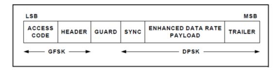
For details, please refer to section 6.5.4.13 in Core\_v5.3, The 3-DH5 packet has between 2 and 1023 information bytes(including the 2-byte payload header) plus a 16-bit CRC code.
