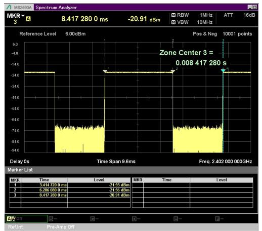
The duty cycle plot is showed above, so the duty cycle of bluetooth is calculated as below:
