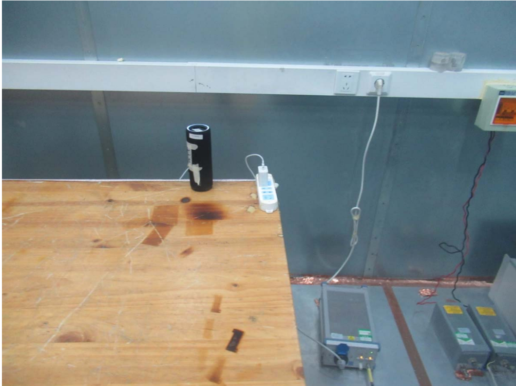
Picture 2 Conducted Emission Test Setup
