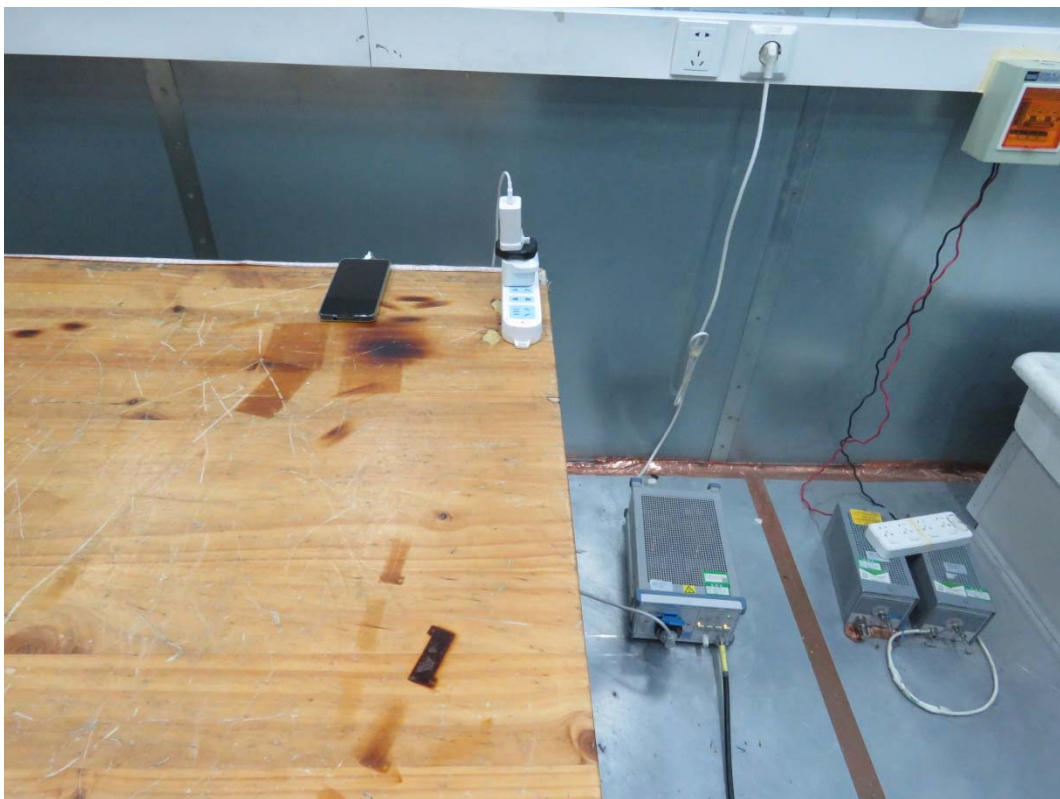
Picture 2 Conducted Emission Test Setup
