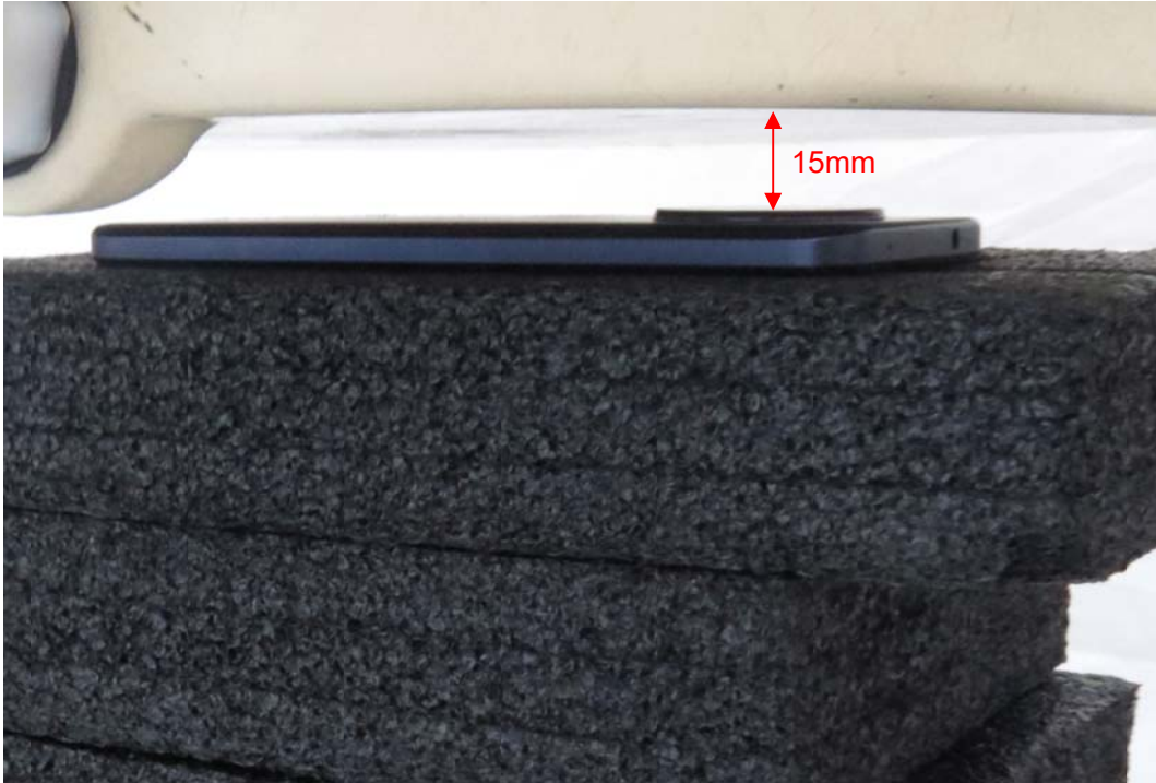
Picture 5: Back Side, the distance from handset to the bottom of the Phantom is 15mm
