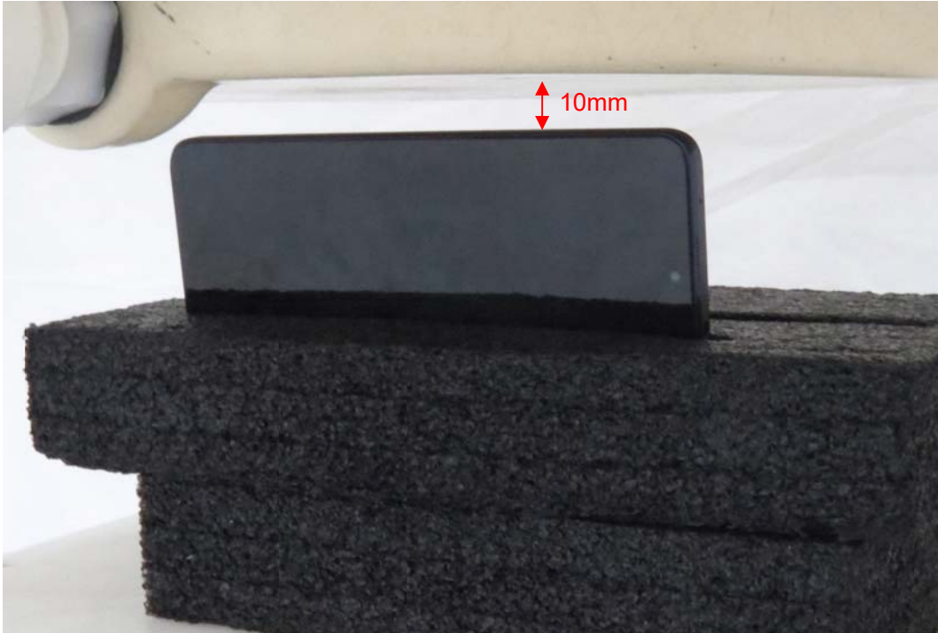
Picture 9: Left Edge, the distance from handset to the bottom of the Phantom is 10mm
