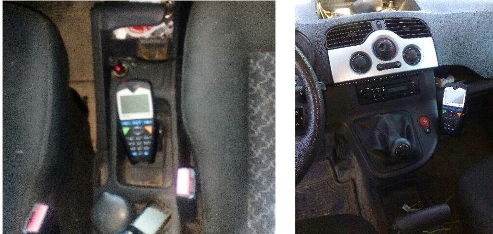
Examples of MCE fastening : MCE BT is powered from cigarette lighter and placed between front seats (top view, left image) ; MCE BT is fastened on storage rack between seats (right image)
