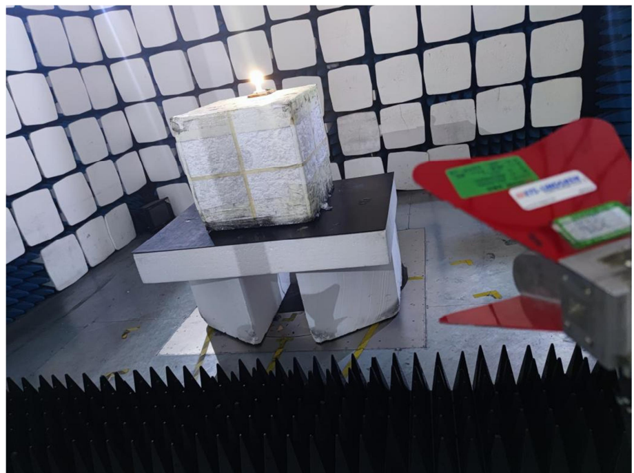
Radiation Emission Test Setup (1GHz to 18GHz)
