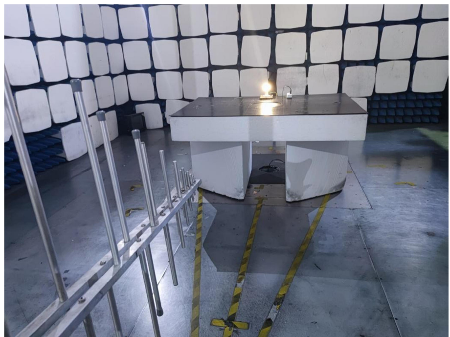
Radiation Emission Test Setup (30MHz to 1GHz)
