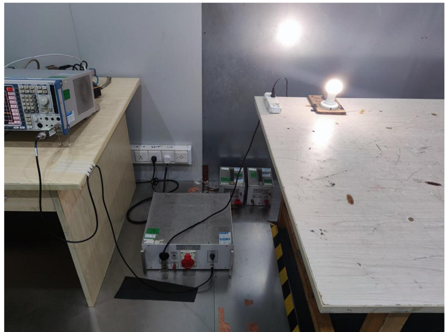
Conducted Emission Test Setup
