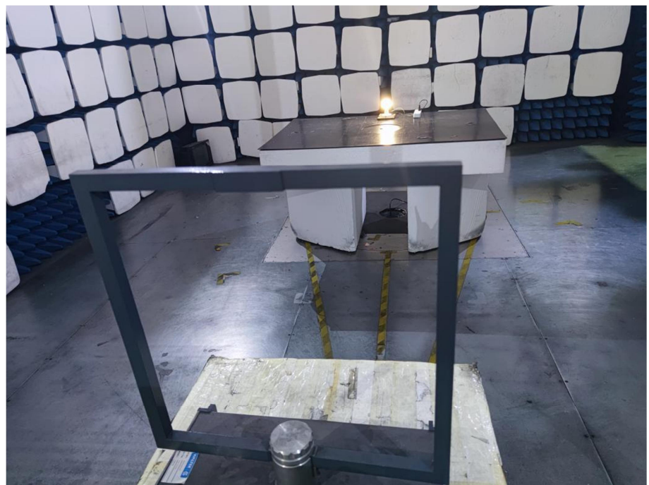
Radiation Emission Test Setup (Below 30MHz)
