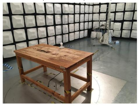
Test Setup For Radiated Emission (Above 1GHz)
