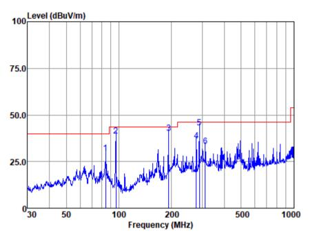
Antenna Polarity :VERTICAL EUT/Project :7293CR Test mode :A
