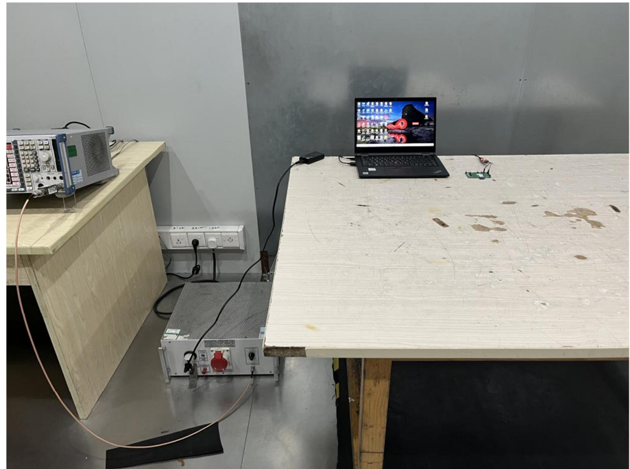
Conducted Emission Test Setup
