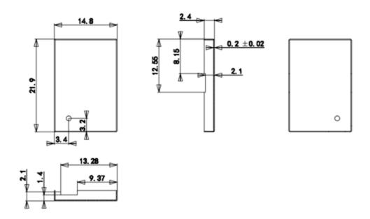
Fig 9 BL3359-P Dimensions of shielding case
