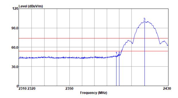
Mode:a; Polarization:Horizontal; Modulation:b; bandwidth:20MHz; Channel:Low
