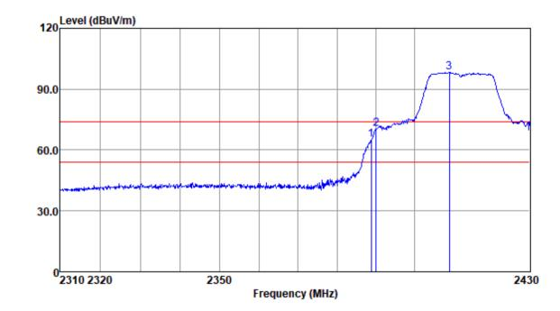
Mode:a; Polarization:Horizontal; Modulation:n; bandwidth:20MHz; Channel:Low
