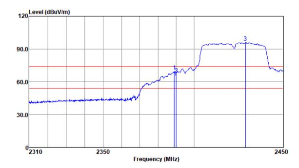
Mode:a; Polarization:Horizontal; Modulation:n; bandwidth:40MHz; Channel:Low
