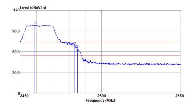
Mode:a; Polarization:Vertical; Modulation:n; bandwidth:20MHz; Channel:High
