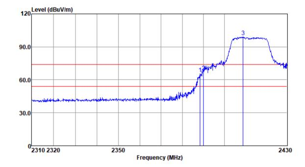
Mode:a; Polarization:Vertical; Modulation:n; bandwidth:20MHz; Channel:Low
