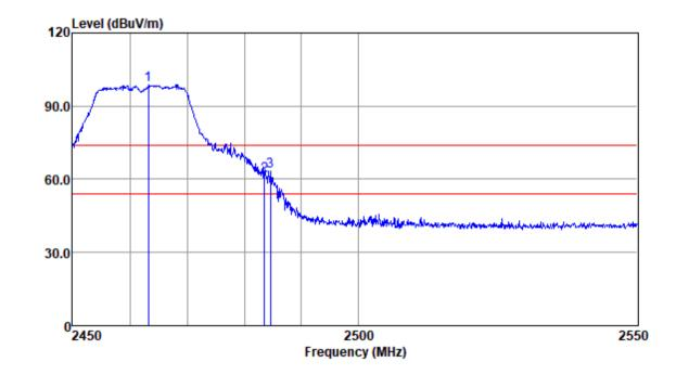
Mode:a; Polarization:Vertical; Modulation:g; bandwidth:20MHz; Channel:High
