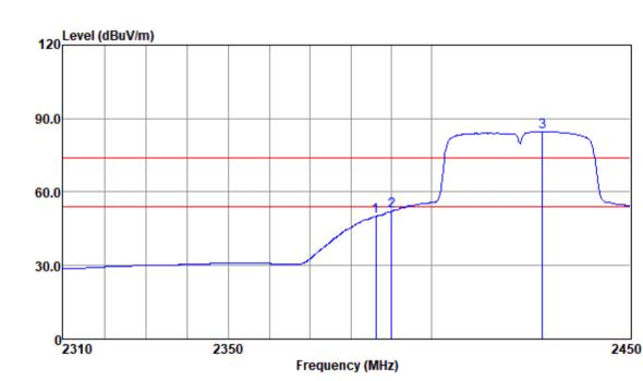
Mode:a; Polarization:Horizontal; Modulation:n; bandwidth:40MHz; Channel:Low
