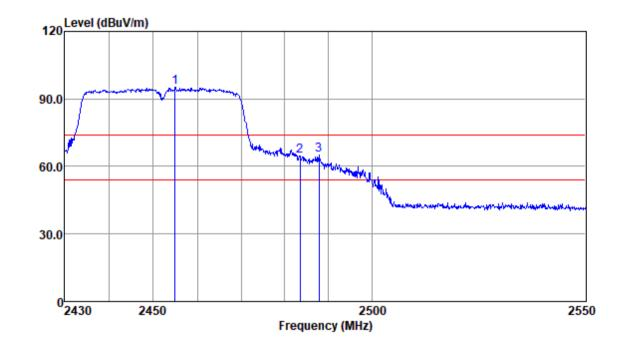
Mode:a; Polarization:Vertical; Modulation:n; bandwidth:40MHz; Channel:High
