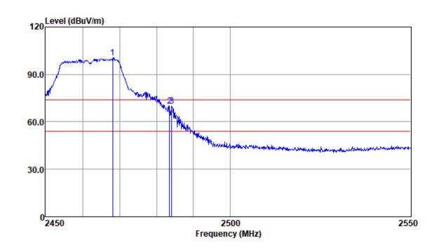
Mode:a; Polarization:Horizontal; Modulation:g; bandwidth:20MHz; Channel:High
