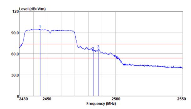
Mode:a; Polarization:Horizontal; Modulation:n; bandwidth:40MHz; Channel:High
