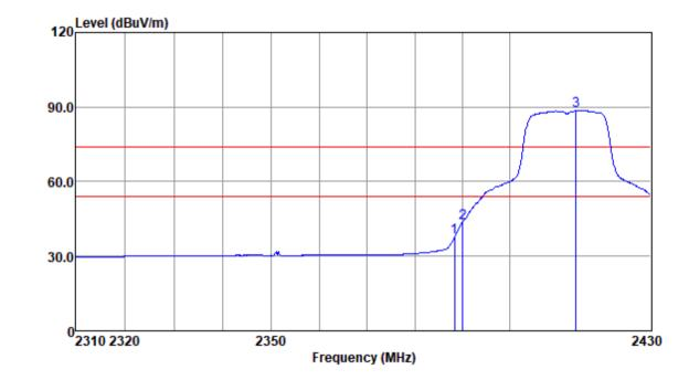
Mode:a; Polarization:Vertical; Modulation:g; bandwidth:20MHz; Channel:Low
