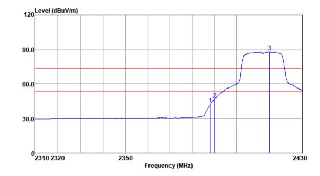
Mode:a; Polarization:Vertical; Modulation:n; bandwidth:20MHz; Channel:Low
