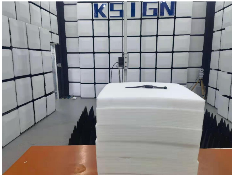
Radiated Measurement (Above 1GHz)
