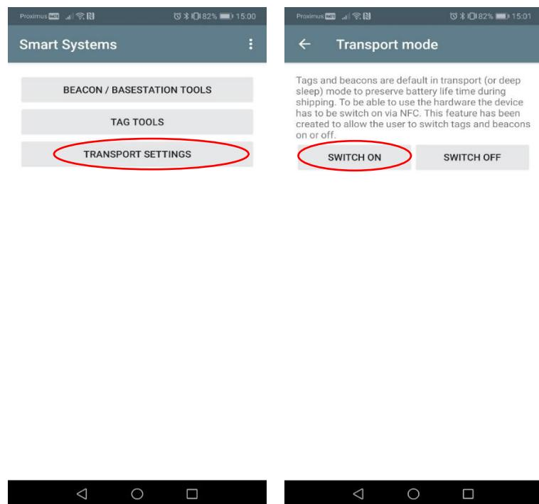
To switch on the device, tap the “SWITCH ON” button and hold the device close the NFC antenna of your smartphone.
