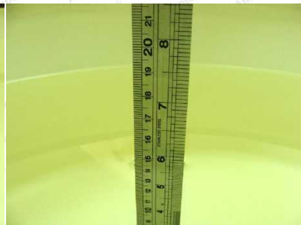
Photo of Liquid Height for Body SAR
