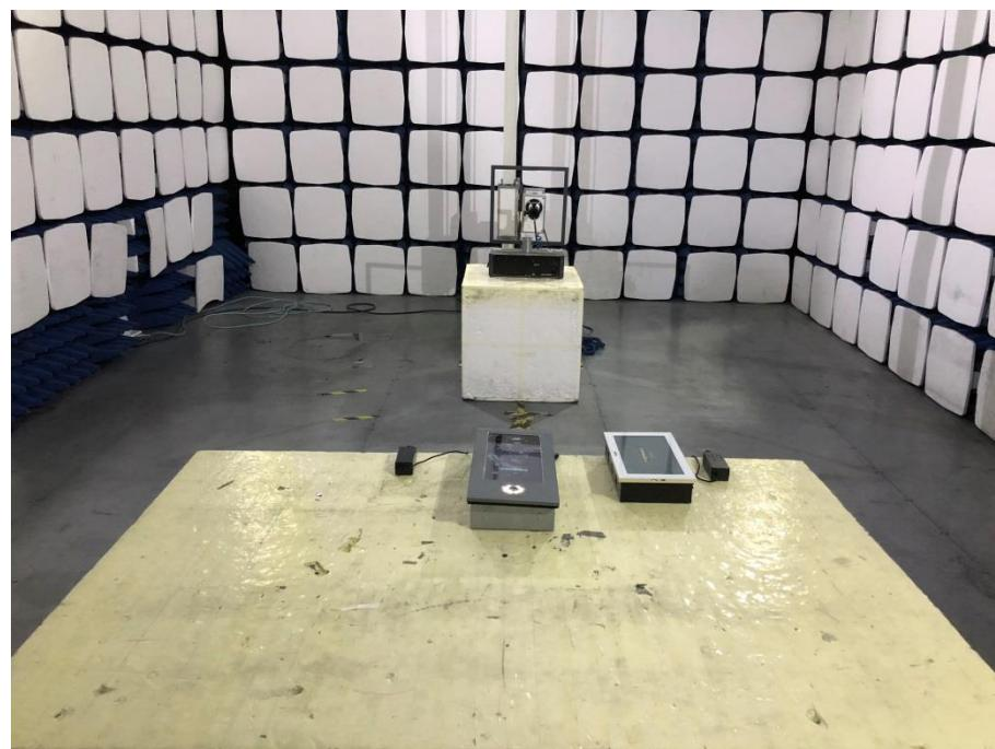
**Radiation Emission Test Setup (30MHz to 1GHz)**
