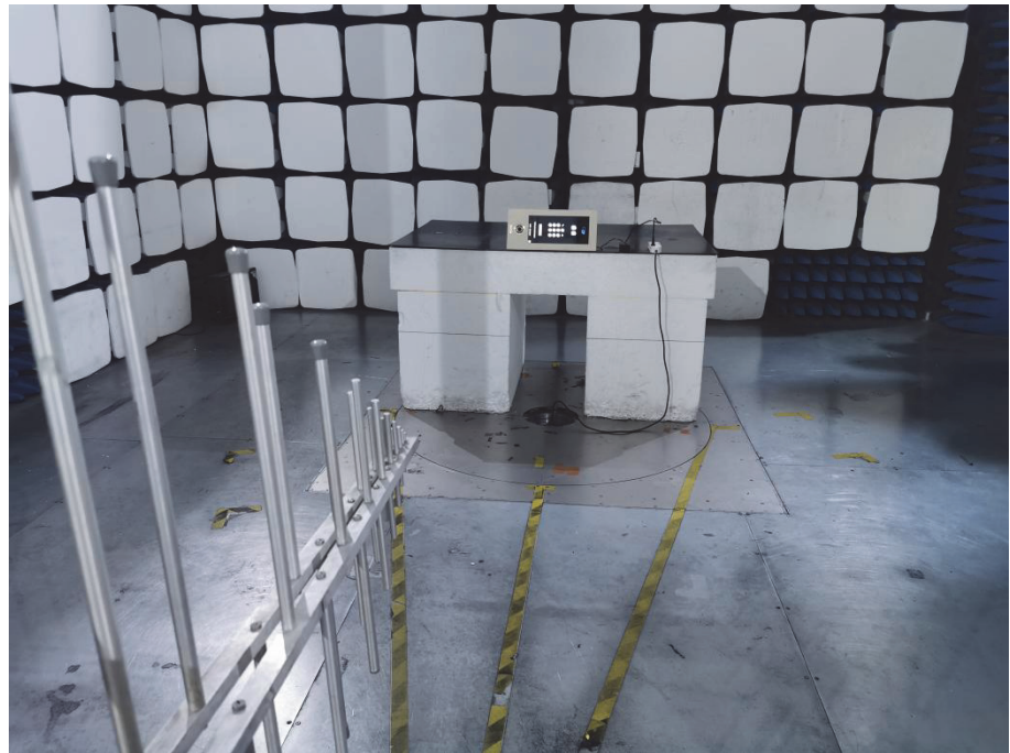
Radiation Emission Test Setup (30MHz to 1GHz)
