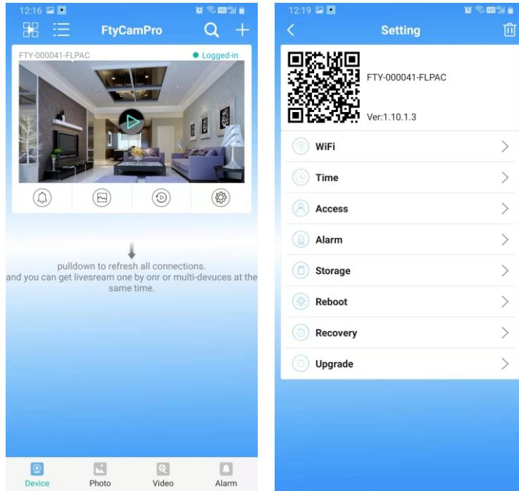
2. Configure the WIFI connection for the camcorder. Select "WIFI setting" to display available Wi-Fi hotspots. Select your Wi-Fi network name (SSID), input the password, and press the "Completion" button. Note: If the camcorder is in WIFI status after being saved, it will disconnect the current connection for a new WIFI network, which will make the camcorder offline for about one minute in the APP.
