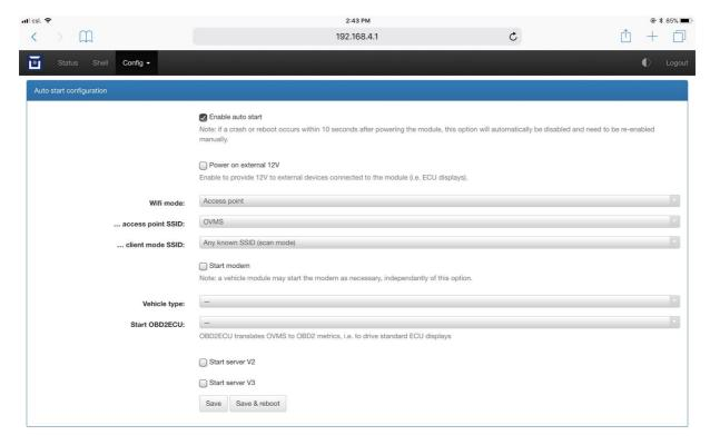
You will usually want to click to "Enable auto start", and "Start server v2". The other fields should have been populated correctly automatically for you. If you are using the optional modem module, you should also click "Start modem" to enable the modem.
