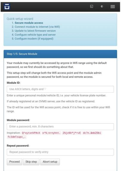
The wizard will need to reconfigure the module for the Wifi setup, read the notes and be prepared to reconnect to the module as necessary.
