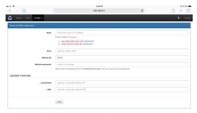
You should enter the server host (api.openvehicles.com, or ovms.dexters-web.de, usually), and vehicle password (aka 'server password' - as entered on the server when you registered your vehicle). The Vehicle ID field should already be there, and the other parameters are optional.
