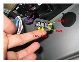
The OVMS Data Cable for Tesla Roadster can then be plugged in, connecting the car to the
