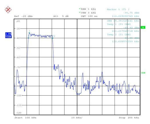
According the test data above, the fundamental wave is not fall in the restricted band 90KHz-110KHz, the field strength also meet the 15.209 requirement, refer to Radiated Emissions (9kHz-30MHz).
