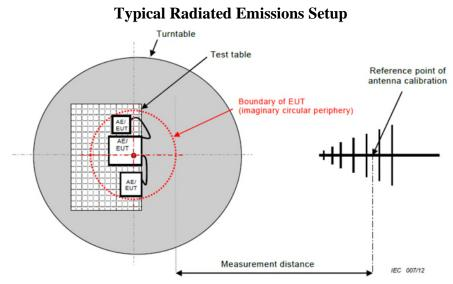
Spurious radiated emission limits are converted from a power limit to a field strength limit at 3 meter. The conversion formula used is dBuV/m = dBm + 104.77 - 20log(R).
